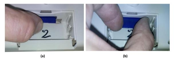
Figure 5. (a) Releasing and, (b) pulling out the SD card.
